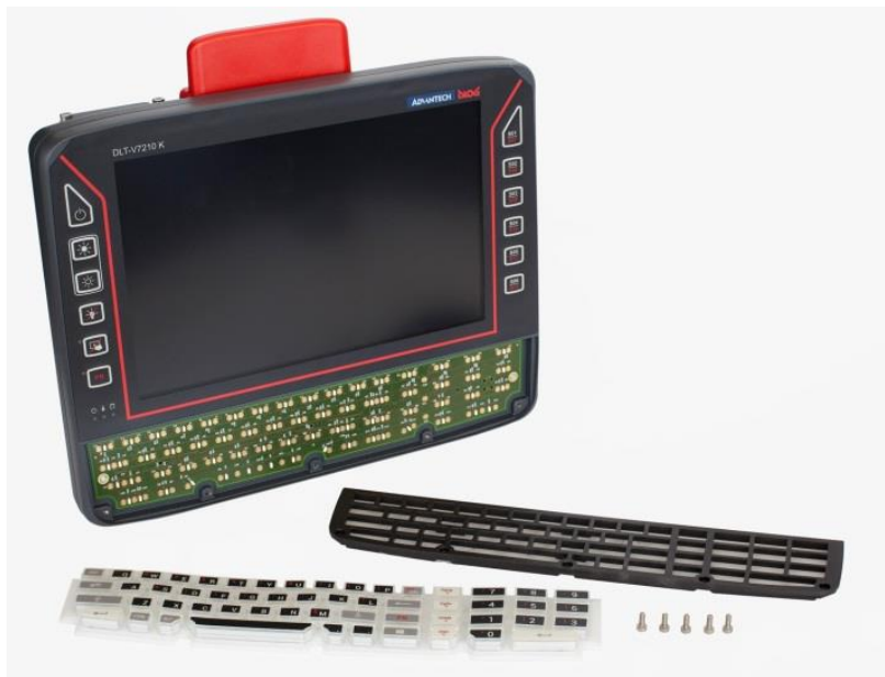
Fig. 16.2: Integrated keyboard: Keyboard components
