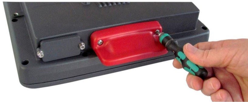
Fig. 7.5: WLAN antenna IEEE 802.11 a/b/g/n/ac
