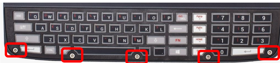
Fig. 16.1: Integrated keyboard: Unscrew the mounting screws
