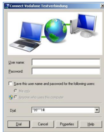
Fig. 11.6: QUECTEL EC25 - Dial Vodafone test connection
