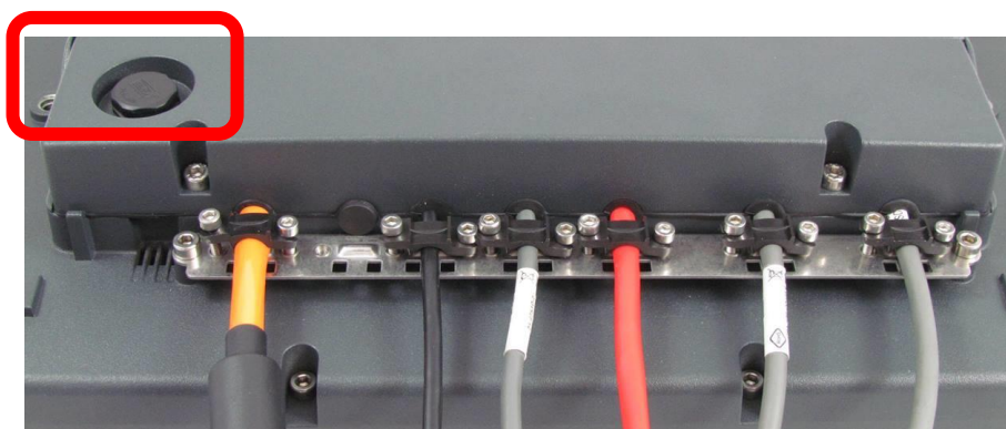
Fig. 13.6: Pressure compensation element
