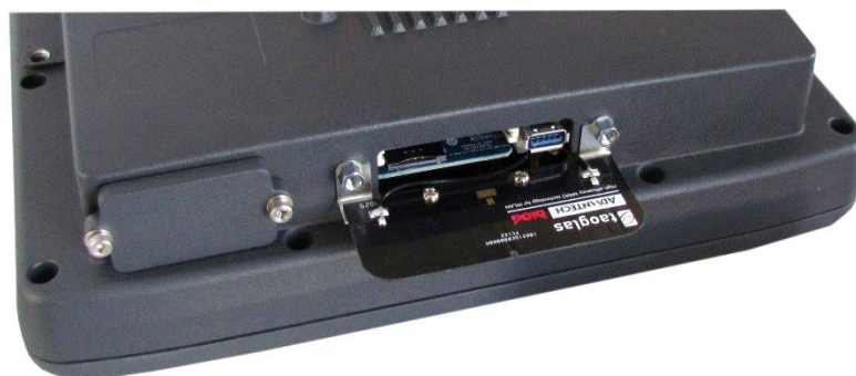
Fig. 7.6: WLAN antenna IEEE 802.11 a/b/g/n/ac opened
