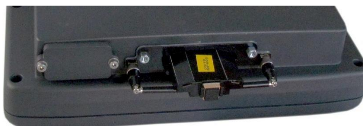
Fig. 7.9: WLAN, WWAN LTE 4G antenna opened
